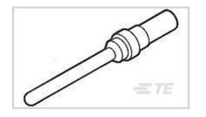
Contact Type: Pin D-Sub Contact Size: 20 Contact Base Material: Copper Alloy Contact Mating Area Plating Material: Gold Termination Method to Wire & Cable: Crimp
